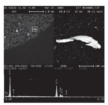
Proper characterization and monitoring of wear debris can provide a prognosis of a components service life.
